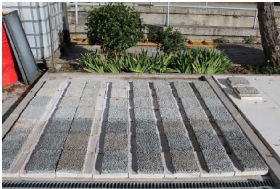
Figure 19: Platform with photocatalytic emulsion applied on one half.
