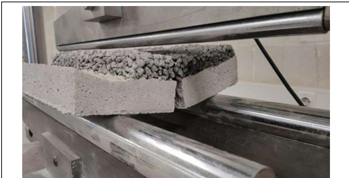
Figure 10: One of the final specimens after breaking in flexure.
