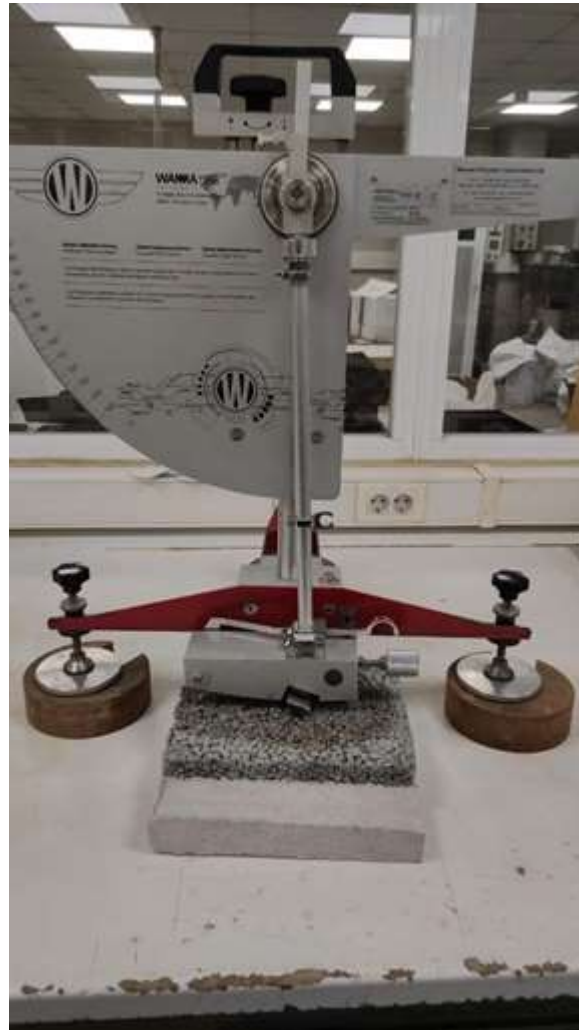
Figure 11: Tile subjected to the slip resistance test.
