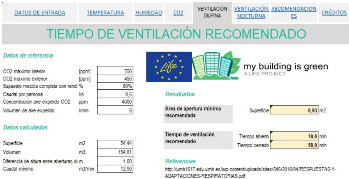
Figure 21. Image of the tool sheet that allows estimating the opening area for ventilation.
