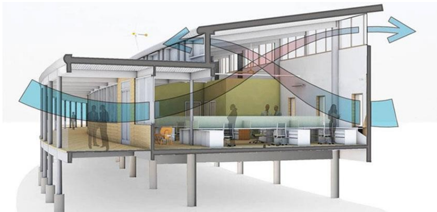
Figure 9. Image illustrating adequate ventilation flows in a building designed with bioclimatic architecture concepts in mind.
