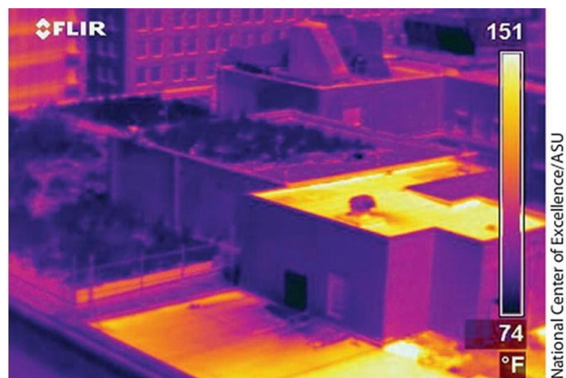
Comparison between the surface temperatures of a green roof and a concrete roof (U.S.EPA, 2008).
