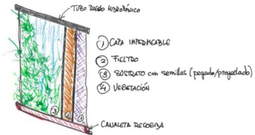
Figure 17. Basic scheme of mBiGToldo.
