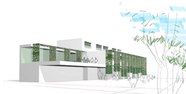
Figure 6: Render of the green wall on the east façade: FAVE system. (Source: Authors’ formulation.)
